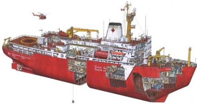
Figure 2-2 Cross-Section of an Icebreaker (Louis St. Laurent)
